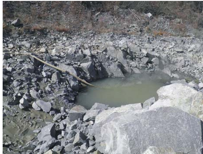
Fig. 17 The amount of ground water in its standpoint 1 was 1.6 m below ground level and in its standpoint Maglovec quarry the amount of ground water levels at the surface blasting
