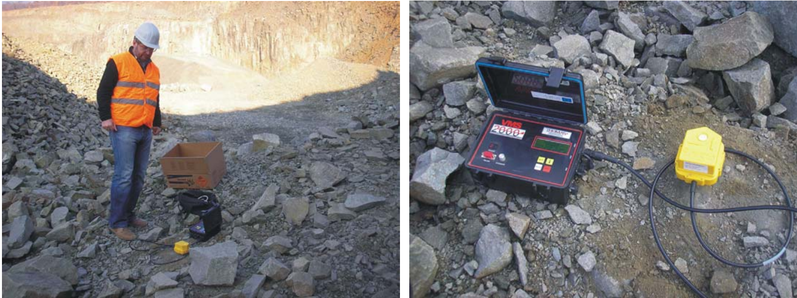
Fig. 8 Measuring position in a I. storey, 20 m from the blast in the Maglovec quarry
