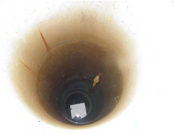
Fig. 17 The amount of ground water in its standpoint 1 was 1.6 m below ground level and in its standpoint Maglovec quarry the amount of ground water levels at the surface blasting
