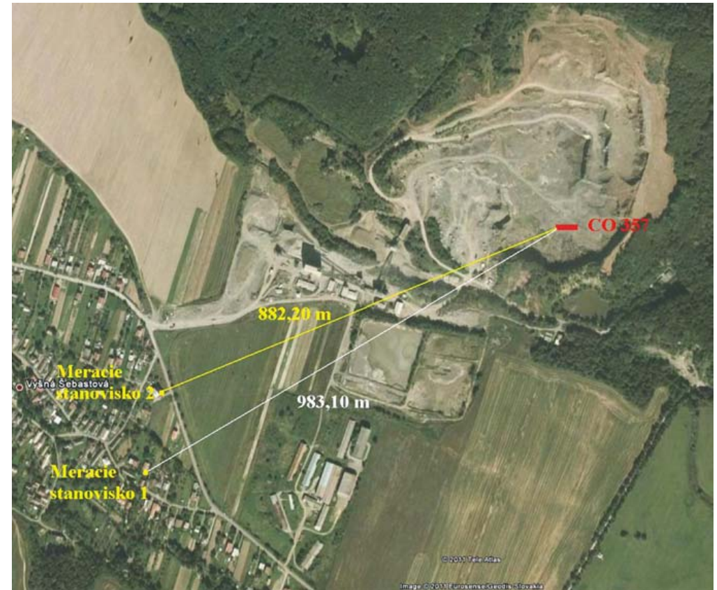
Fig. 3 Measuring position 1 and 2 family house No. 255 in the village Vyšná Šebastová and panel house No. 218 and their position to blasting
