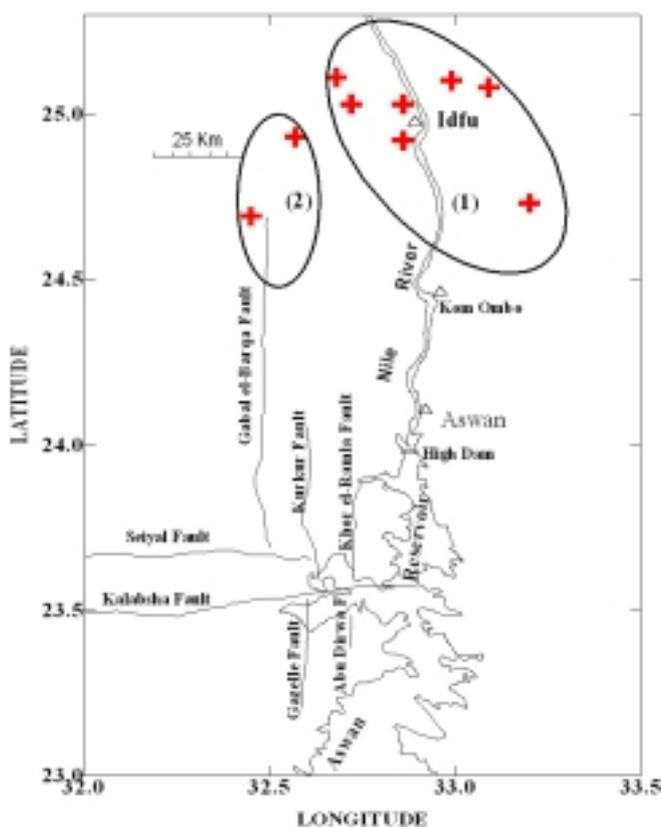
Fig 3 The main significant faults in Aswan region (After WWCC, 1985), and the epicentral distribution of the seismic activity in the study area during the period 1982 – 2006.
