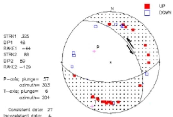
Fig. 4 Focal mechanism solution of the Dec. 13, 2006 earthquake.
