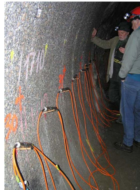
**Fig. 1** The placing of the electrodes on the Bedřichov gallery wall
