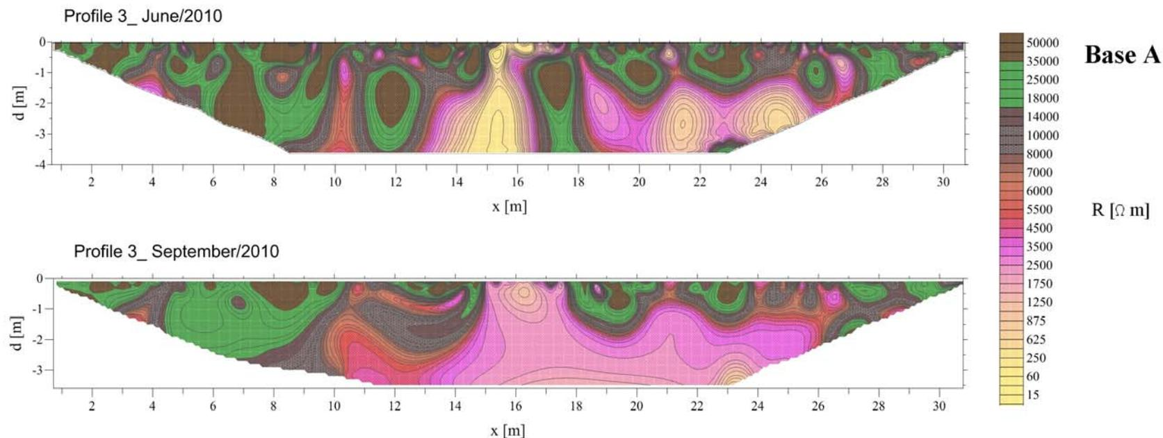
**Fig. 2** The comparison of resistivity cross sections from June and September 2010 at base A
