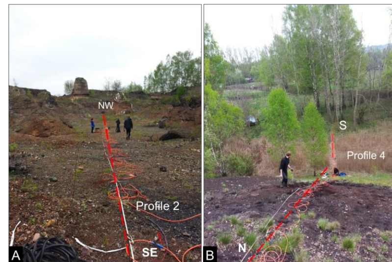
Fig. 2 Location of the ERT profiles on the part of waste dump partly exploited (A) and on the boundary between the waste dump and surrounding clayey soils (B)
