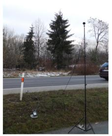
Fig. 9 Measuring reference point V1 on distance 7.5 m from CTL
