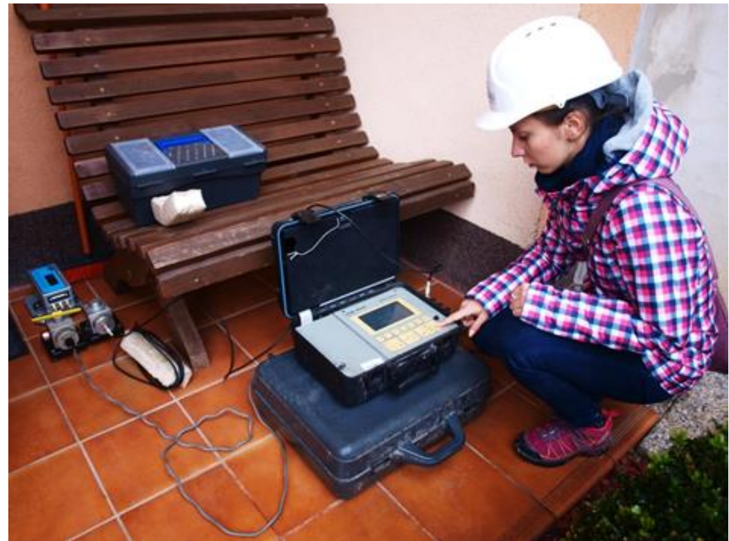
Fig. 6 Position of the seismographs UVS 1504 and ABEM Vibraloc, standpoint S3 (residential building) at a distance of 753.4 m; the first bench blasting CO 643 and at a distance of 657.9 m from the second bench blasting CO 644 in the village Trebejov
