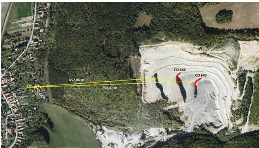
Fig.3 Position and distance of measurement standpoint S3 from bench blasts CO 643 and from CO 644
