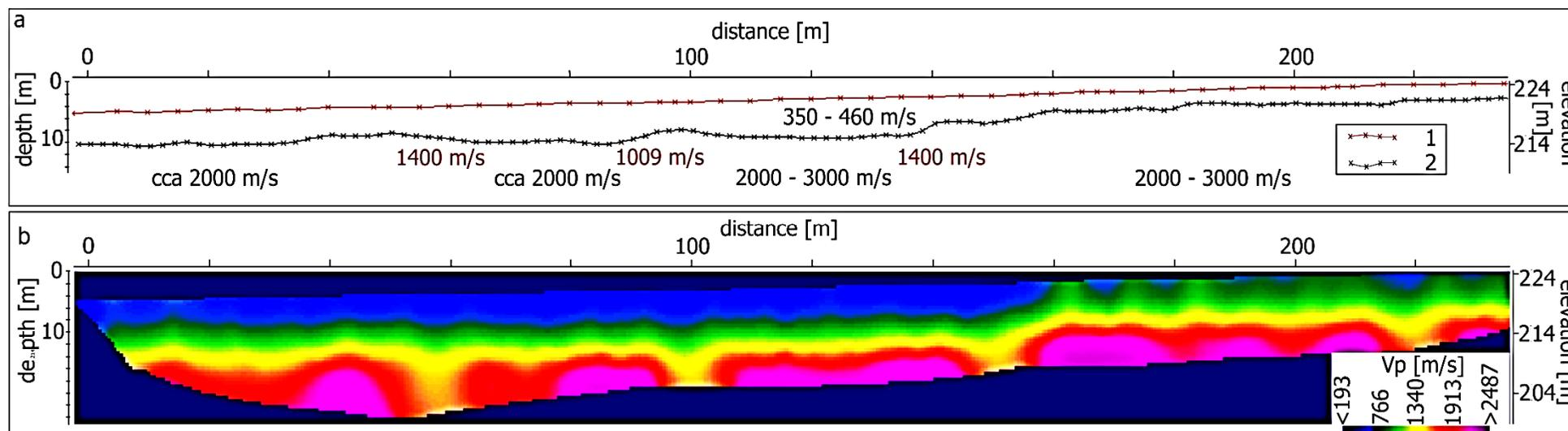
**Fig.3 (a) Refraction seismic measurements – the velocity model, 1 – tomography, 2 – velocity interface; (b) Seismic refraction tomography – the velocity profile.**
