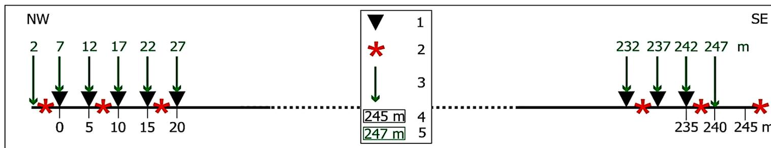
**Fig.2 Sampling point distribution pattern for radon emanometry and seismic line; 1 – position of geophone, 2 – position of source, 3 – position of radon soil sample, 4 – meters distribution for refraction seismic profile, 5 – meters distribution for radon emanometry profile**
