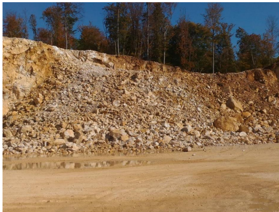
Fig. 13 Rubble after the bench blasting 561 in the quarry Mníchová Lehota
