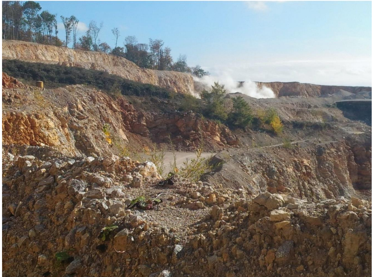
Fig. 3 A view of the individual floors of the quarry Mníchová Lehota with a visible high rate of rock mass disturbance and the site of blasting works
