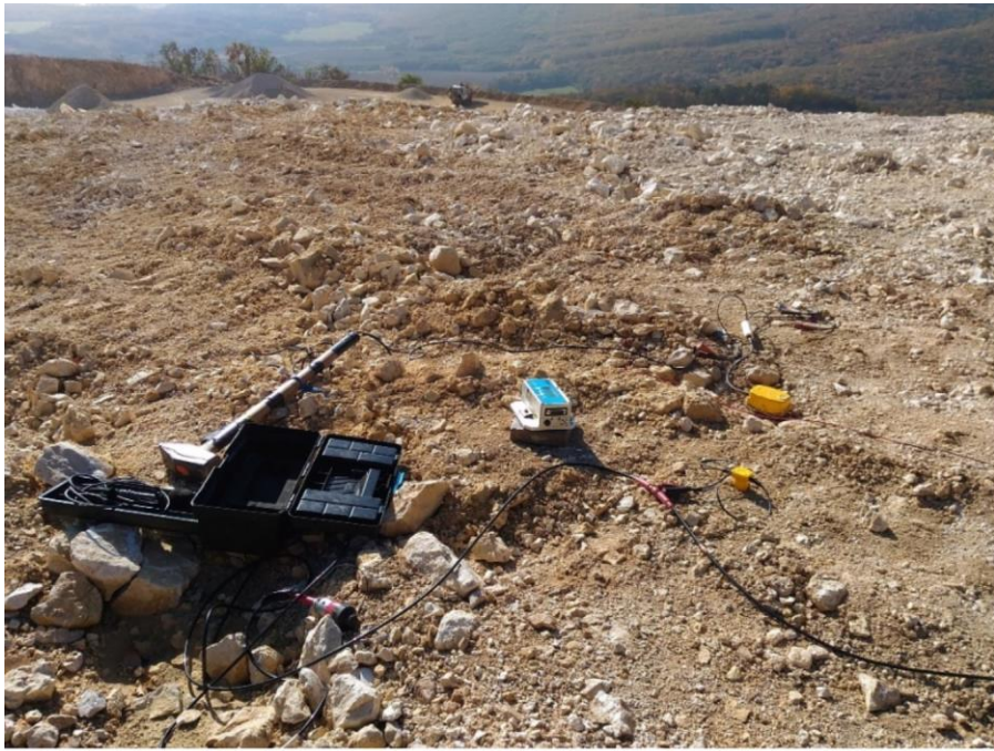
Fig. 4 The monitoring station in the quarry Mníchová Lehota quarry at a distance of 18.5 m from the initial blasthole including the three-component Vibraloc sensor on a special base
