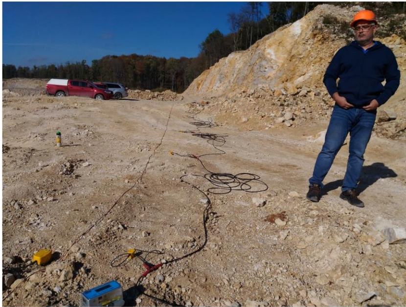
Fig. 8 Seismic profile on the quarry wall before blasting. 24 geophones were deployed in a range of 2 m to the distance of 48 m
