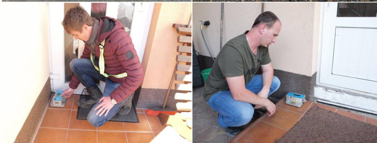
Fig. 5 Apparatus ABEM Vibracloc for measuring the particle velocity of the seismic waves, placed in the front part of the house - entrance to the housing object No. 21 in the village Trebejov - standpoint S2. The standpoint S3 position was at the entrance to the back of the house
