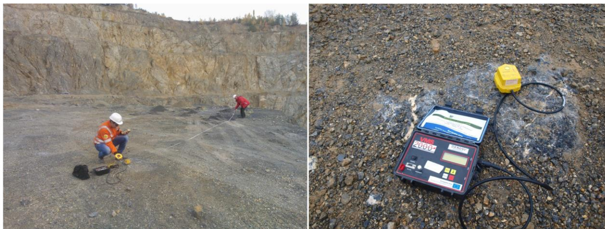
Fig. 4 Position of the seismic apparatus MS 2000 MP at measuring the blasts, standpoint S1 in Trebejov quarry
