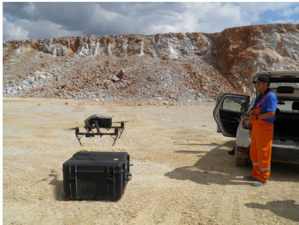
Fig. 1 3D scanning the fresh rock fragmentation during bench blast a drone in a quarry
