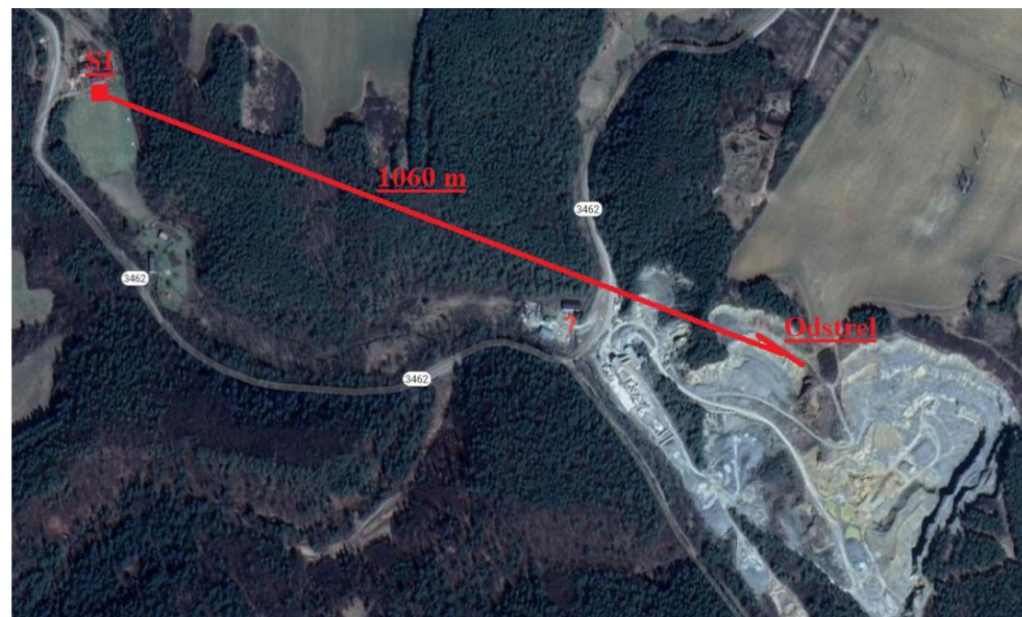
Fig. 5 Position and distance between bench blasting in Sedlice quarry and position of measurement at house in Sedlice village.
