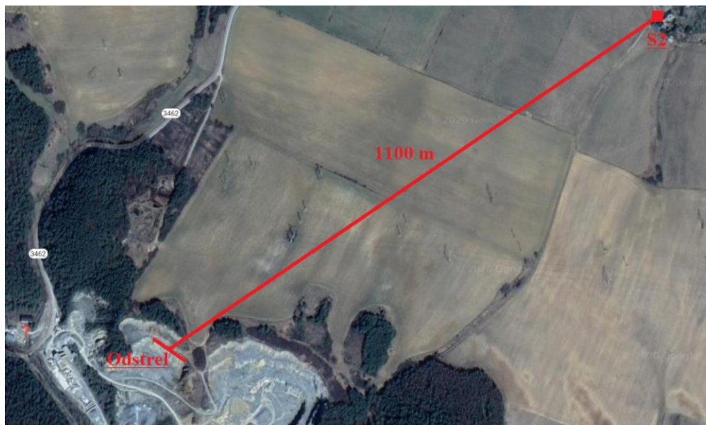
Fig. 4 Position and distance between bench blasting in Sedlice quarry and position of measurement at house in Miklušovce village.
