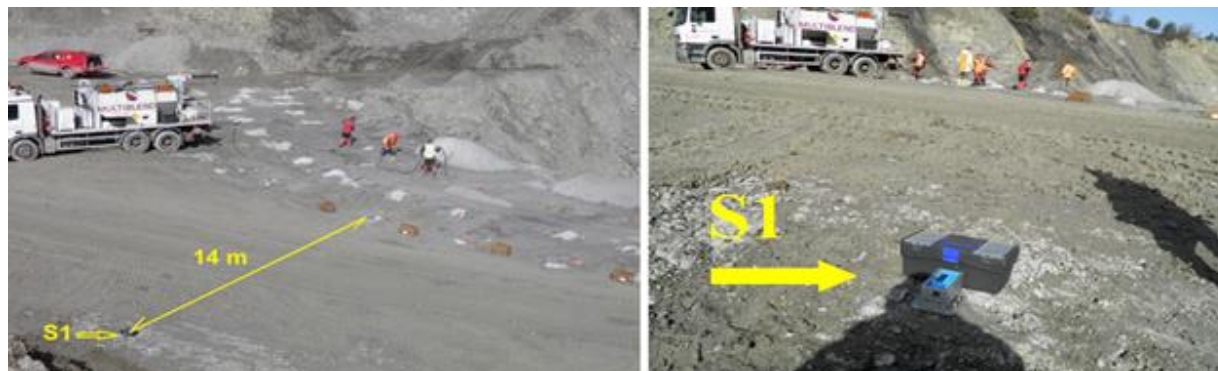
Fig.6 Measuring position S1 (14 m from the initial borehole) and the used measuring vibrograph ABEM Vibraloc placed on the rock
