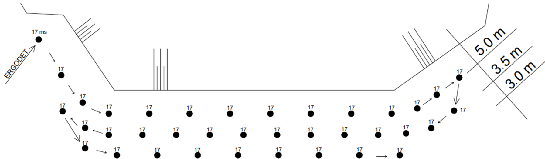
Fig. 14 Scheme of millisecond timing and distribution of boreholes during three-row bench blast CO 143 in Lietavská Lúčka quarry
