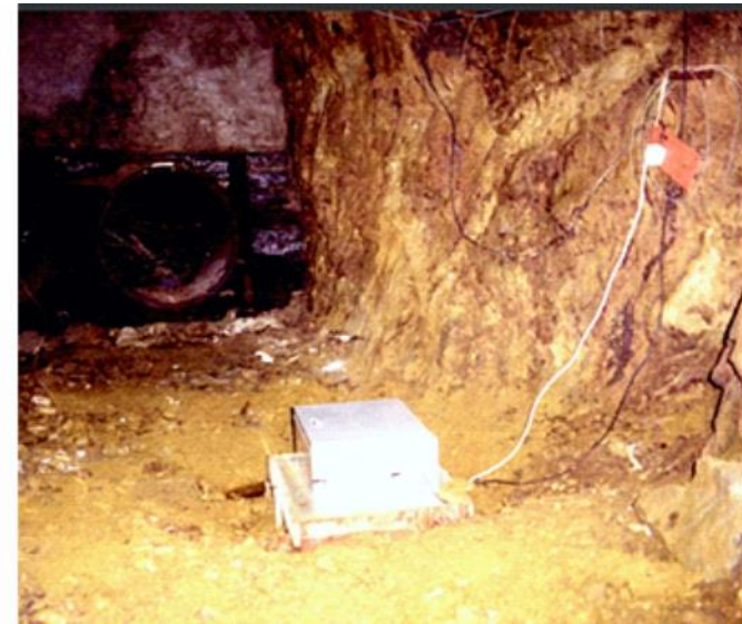
Fig. 4 Entrance to the Subterranean Spaces of Sanatorium EDEL Ltd. in 2003 (left) and seismic pillar with a case with seismometers and remote telemetric transmitter (photo: Kaláb)
