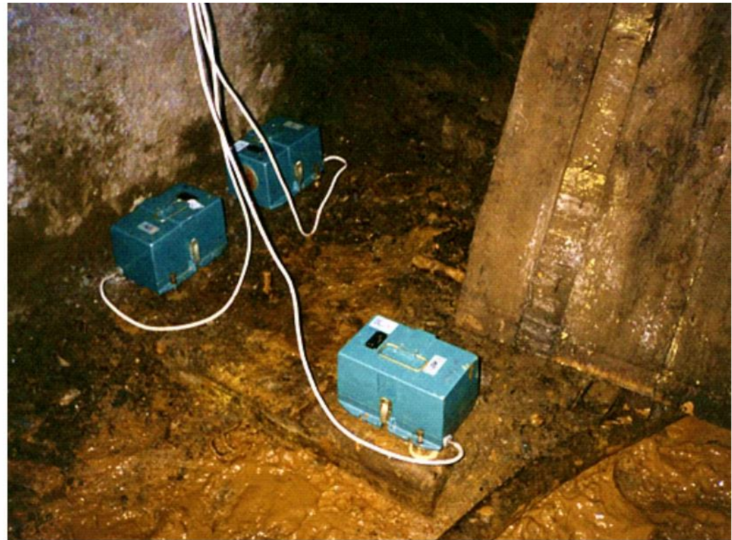
Fig. 3 Seismic apparatus PCM3-EPC located in the engine room on the surface (left) and three seismometers SM-3 located on the third level of the mine (right) – photos: Kaláb
