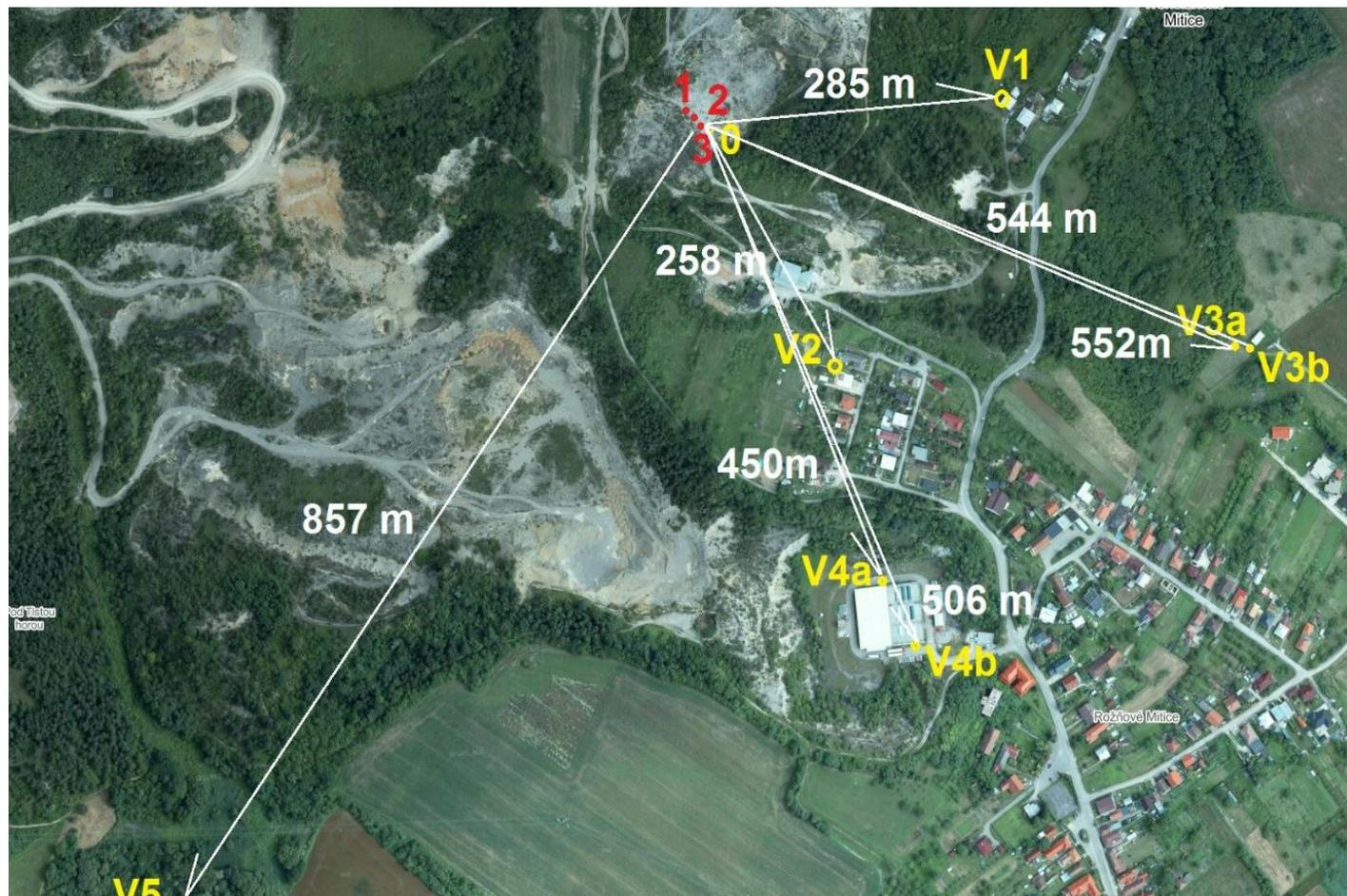
*Fig. 1 The positions of test blasts 1, 2 and 3 in the quarry Trenčianske Mitice Skaličky in relation to measuring standpoints 0 to 7 located in the vicinity of the quarry*
