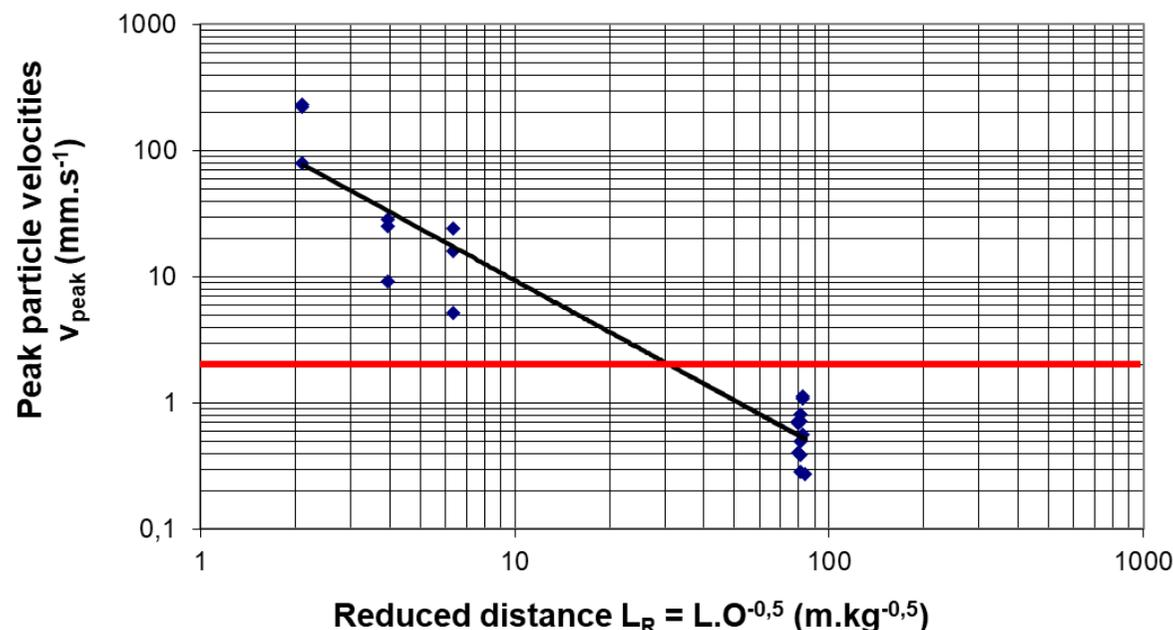
**Fig. 8** *Seismic waves attenuation law for the quarry Trenčianske Mitice Skalničky and water source Zadná studňa spring in the village Trenčianske Mitice.*
