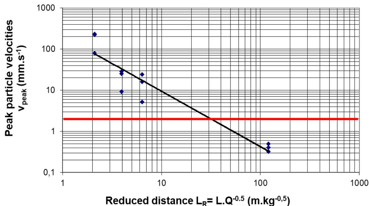
*Fig. 9 Seismic waves attenuation law for the quarry Trenčianske Mitice Skalničky and mineral water source MP – 1 nearby the village Trenčianske Mitice.*
