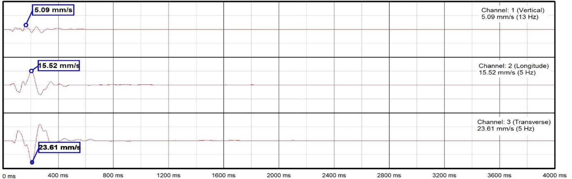
**Fig. 7** *Graphic record of the individual components of seismic waves in the quarry Trenčianske Mitice Skaličky. The recording is from the vibrograph Vibracord at the measuring standpoint V0, 45 m from the initiation borehole of blast No. 1.*
