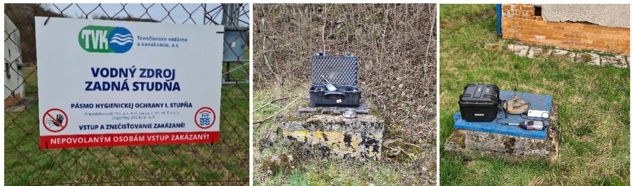
**Fig. 3** Measuring standpoints V3a and V3b water source Zadná studňa spring and pump and vibrographs Svantek with sensors
