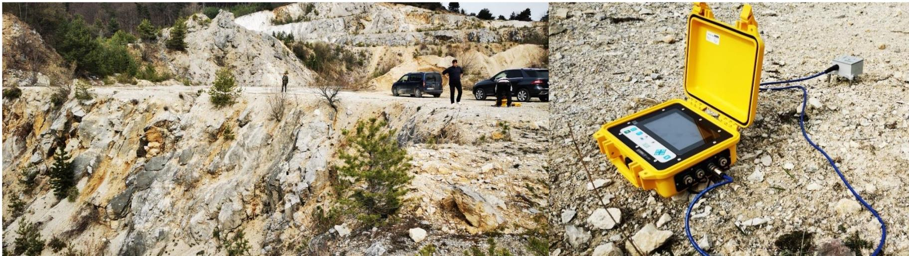
**Fig. 2** Measuring standpoint V0 quarry Trenčianske Mitice - Skalníčky and vibrograph Vibracord with a three-component geophon at a distance of 15 m from the initiation borehole of blast No. 3
