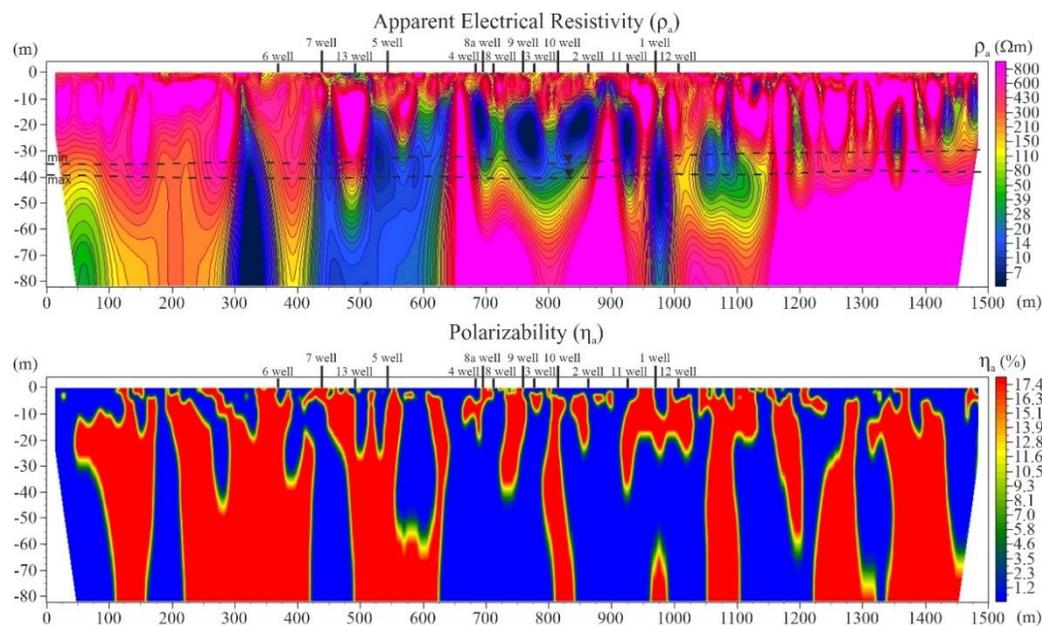
**Fig. 5** *Electrotomographic section along the profile I – I. Min and max boundaries are the intervals of fluctuations in groundwater levels (GWT)*
