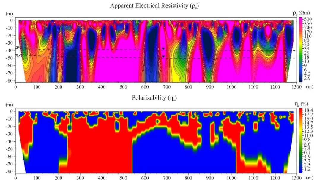
**Fig. 7** *Electrotomographic section along profile III – III. Min and max boundaries are the intervals of fluctuations in groundwater levels (GWT)*
