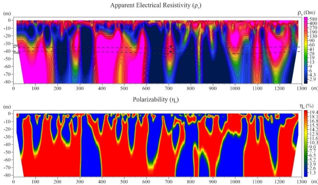
**Fig. 8** *Electrotomographic section along the profile IV – IV. Min and max boundaries are the intervals of fluctuations in groundwater levels (GWT)*
