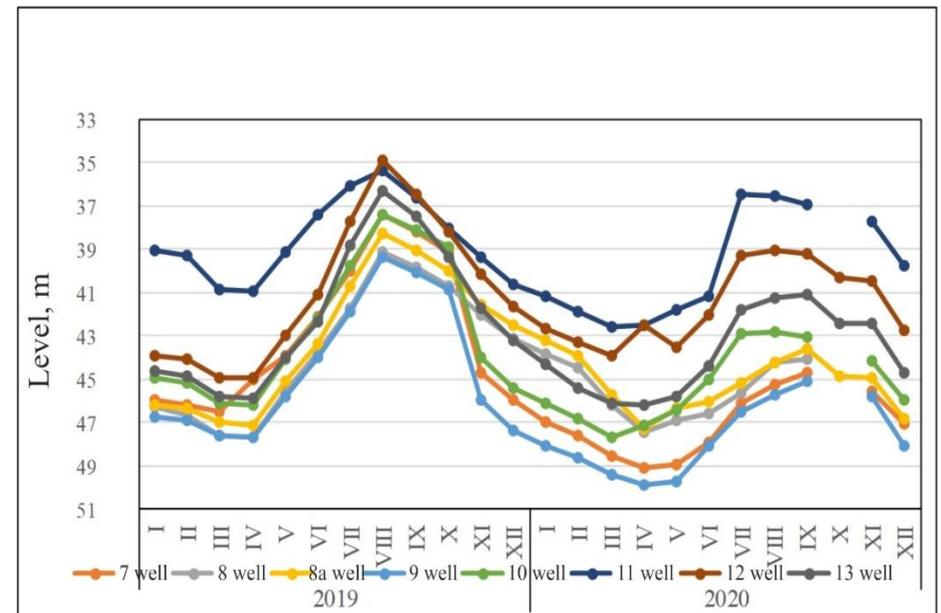
**Fig. 4** *Seasonal changes in the groundwater level for observation wells in the industrial site. Level, m - means meters below the surface of the earth*
