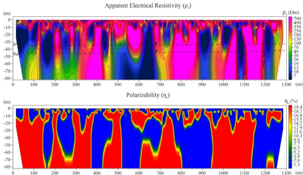
**Fig. 6** *Electrotomographic section along the profile II – II. Min and max boundaries are the intervals of fluctuations in groundwater levels (GWT)*
