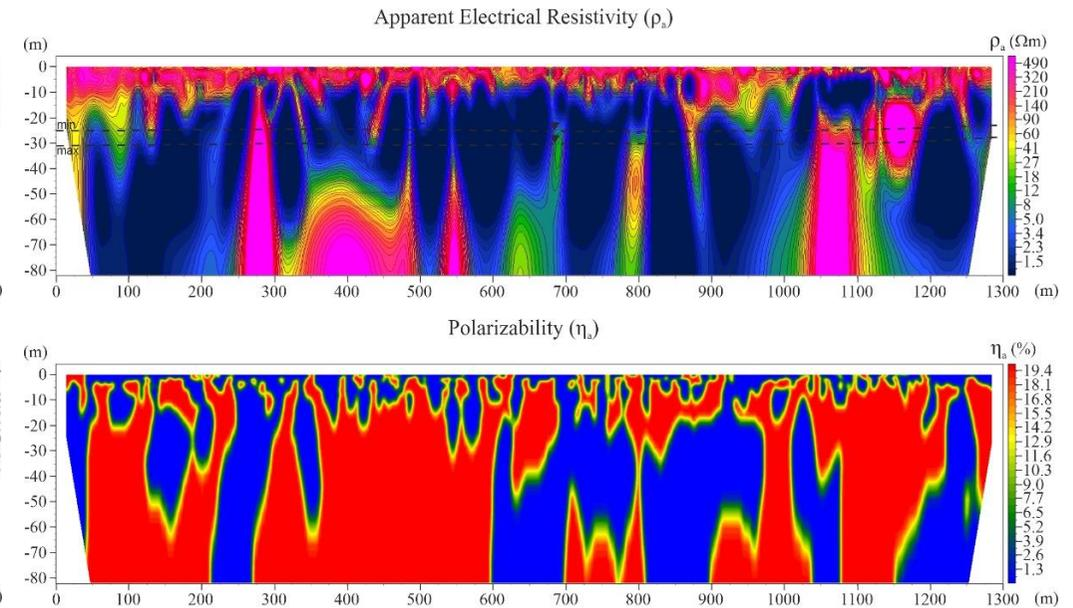
**Fig. 9** *Electrotomographic section along the profile V – V. Min and max boundaries are the intervals of fluctuations in groundwater levels (GWT)*
