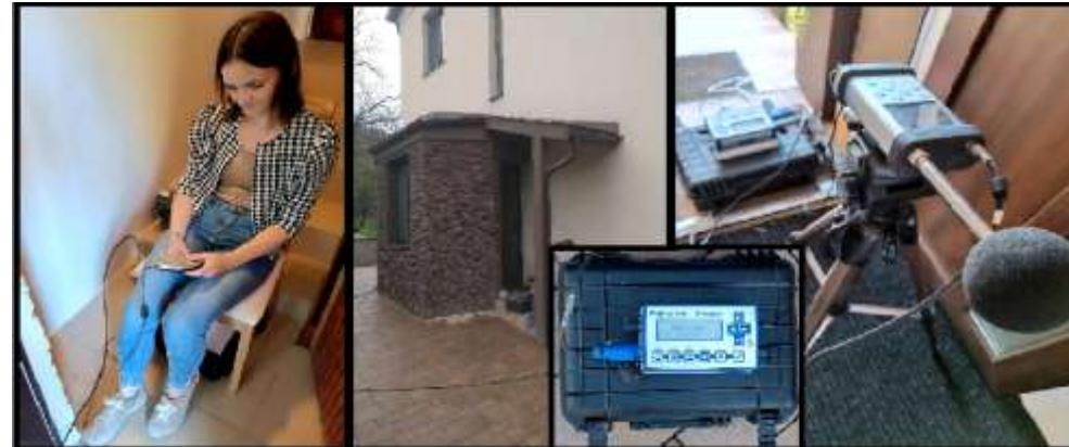
Fig. 6 Measuring standpoint MS 2 and position of measuring instruments in the monitored residential building in the village of Slanec at a distance of 1872 m from the blasting in the quarry Slanec
