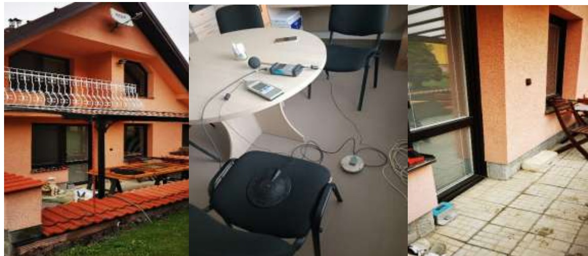
Fig. 10 Measuring standpoint MS 1 and MS 2. Position of measuring instruments at the monitored residential building in the village of Seveřná at a distance of 445 m from the bench blasting in Maglovec quarry
