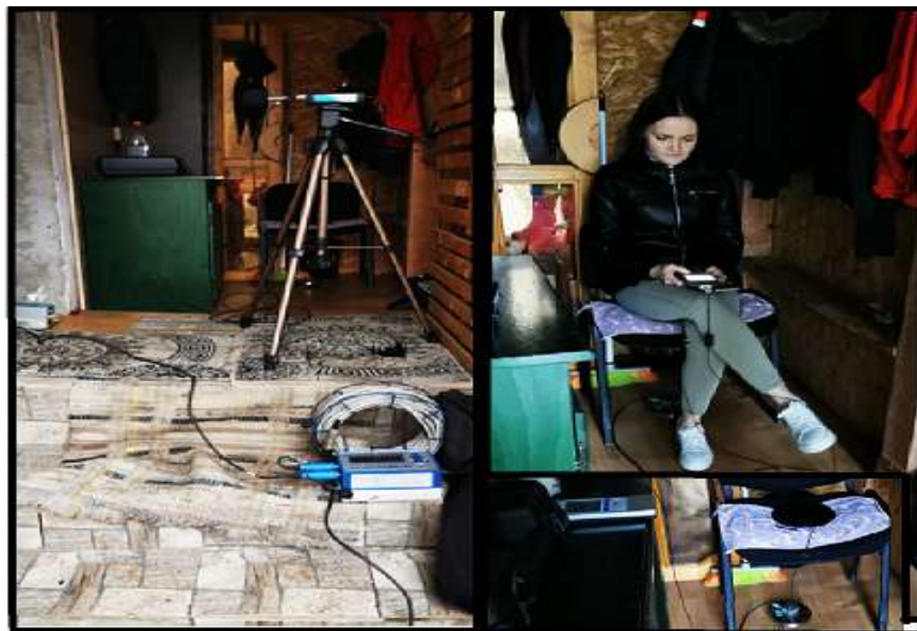
Fig. 4 Measuring standpoint MS 2 and position of measuring instruments in the monitored residential building No. 218 in the village of Nižný Hrabovec at a distance of 417 m from the research blastings
