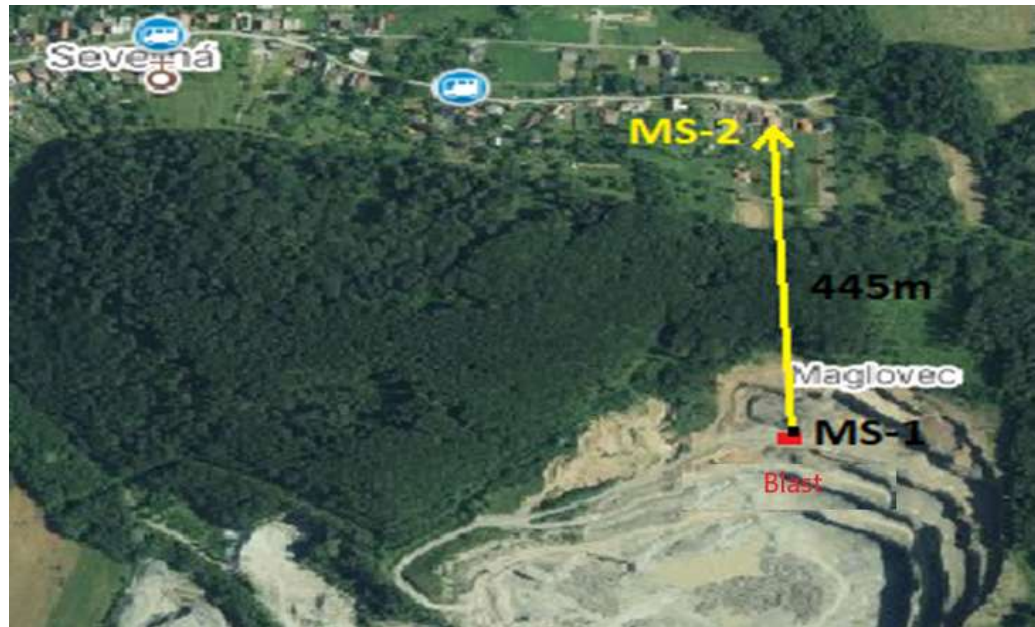
Fig. 9 Position of measuring standpoint MS 1 and MS 2 of blasting in the quarry Maglovec
