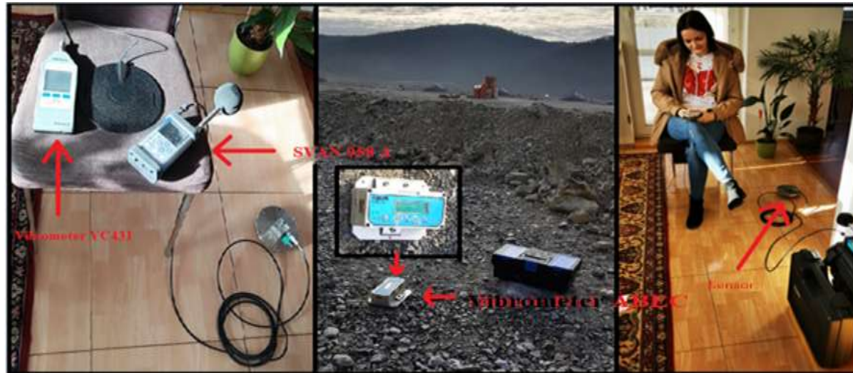
Fig. 8. Measuring standpoint MS 1 and MS 2. Position of measuring instruments in Trebejov quarry and the monitored residential building in the village of Trebejov at a distance of 669 m from the blasting
