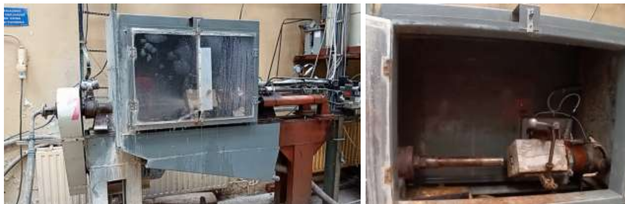
Fig.1 Experimental laboratory horizontal drilling rig (left) and detail of sample holder and drilling tool (right)
