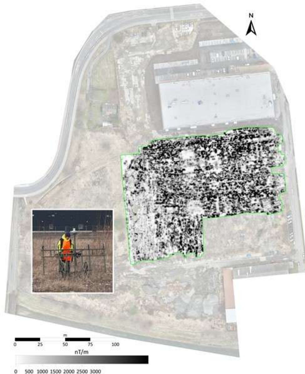
Fig. 3: Map of the analytical magnetometric response across the area of the former foundries with an example measurement using the SENSYS MAGNETO MXPDA device with five fluxgate probes.
